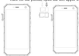
inserted the card slot inside the round hole. Remove the card seat. Fit SIM card to the SIM seat. with the metal surface downward and the edge and corner of the card fitting with the card slot. Slide the SIM card
