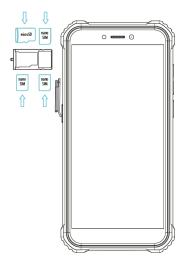
1. Remove the tray that has SIM and microSD cards installed. For removing SIM tray use SIM extractor tool
